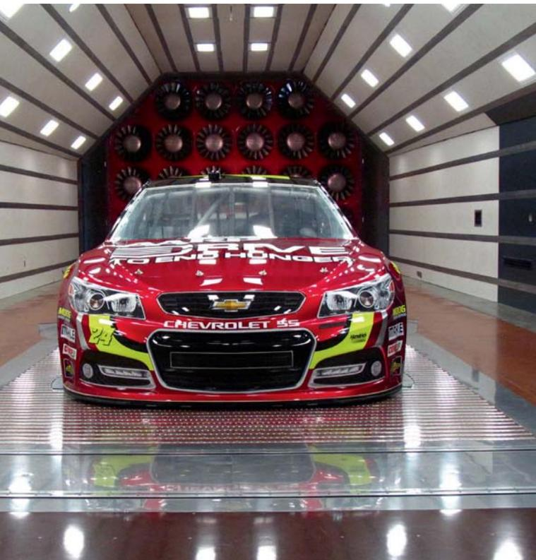
A Generation 6 Chevrolet being put through its paces at the Aerodyn facility in Mooresville, NC - a tunnel that was purpose-built for stockcars
