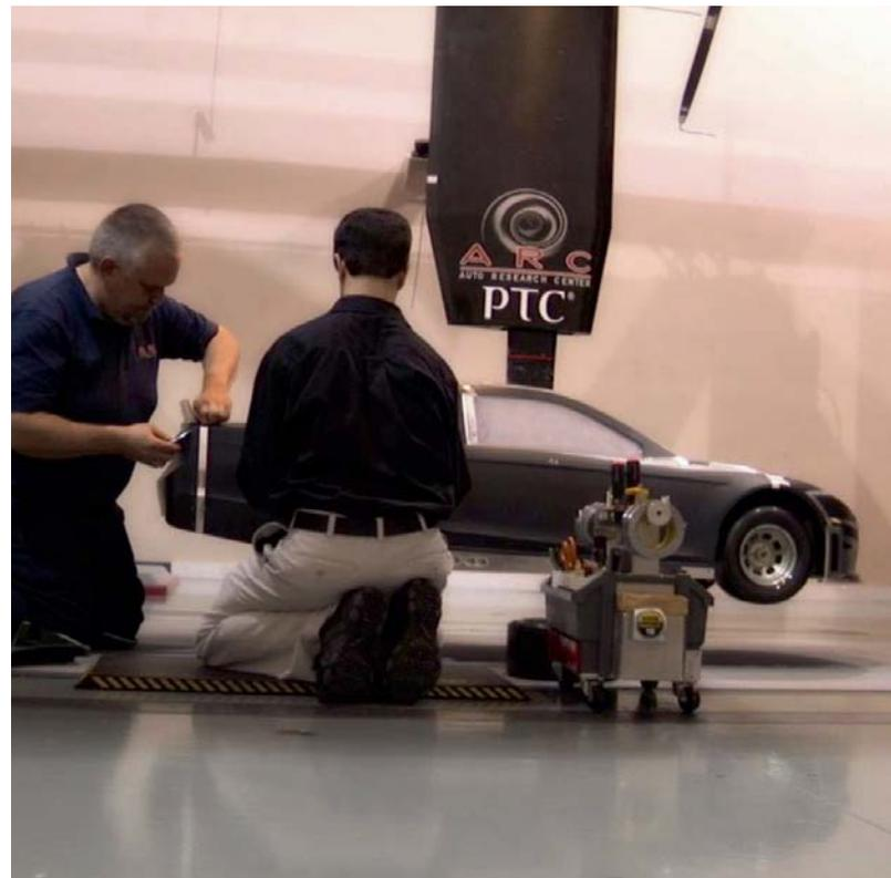
Engineers working on a Generation 6 Ford in the ARC tunnel in Indianapolis - one of only two scale model wind tunnels used regularly by Cup teams
