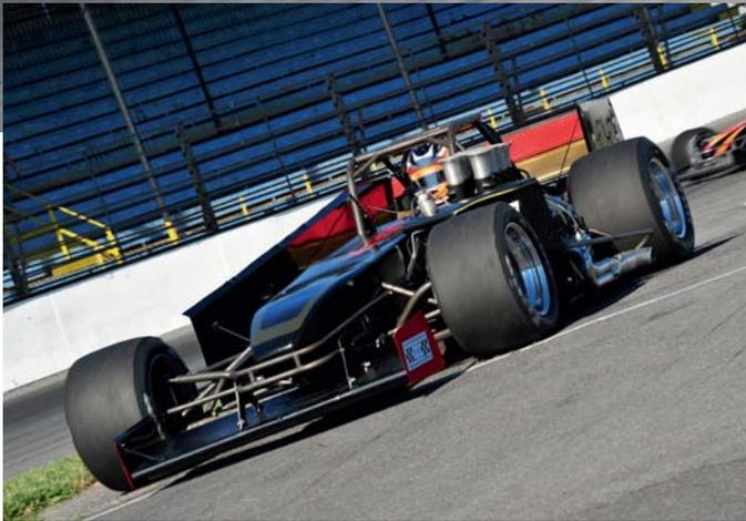
**The cars feature no transmission or gearbox, and the engines drive the rear wheels directly. If a driver spins, that spells the end of their race**
