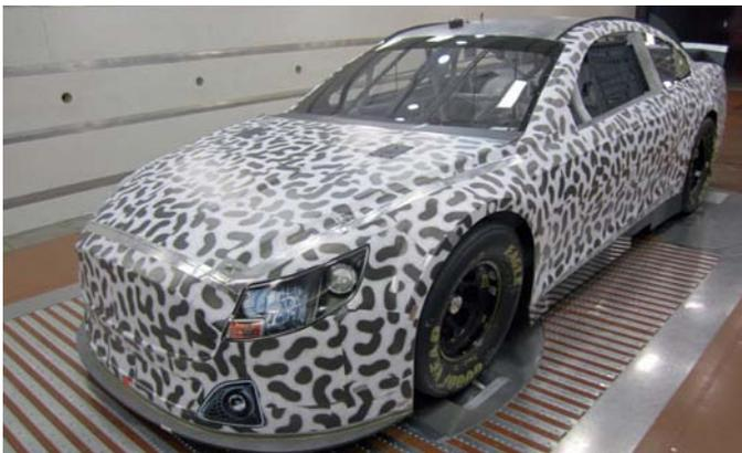
**A Ford in the Aerodyn tunnel, a facility which boasts 22 fans compared to one big fan found in many other wind tunnels, speeding testing up**
